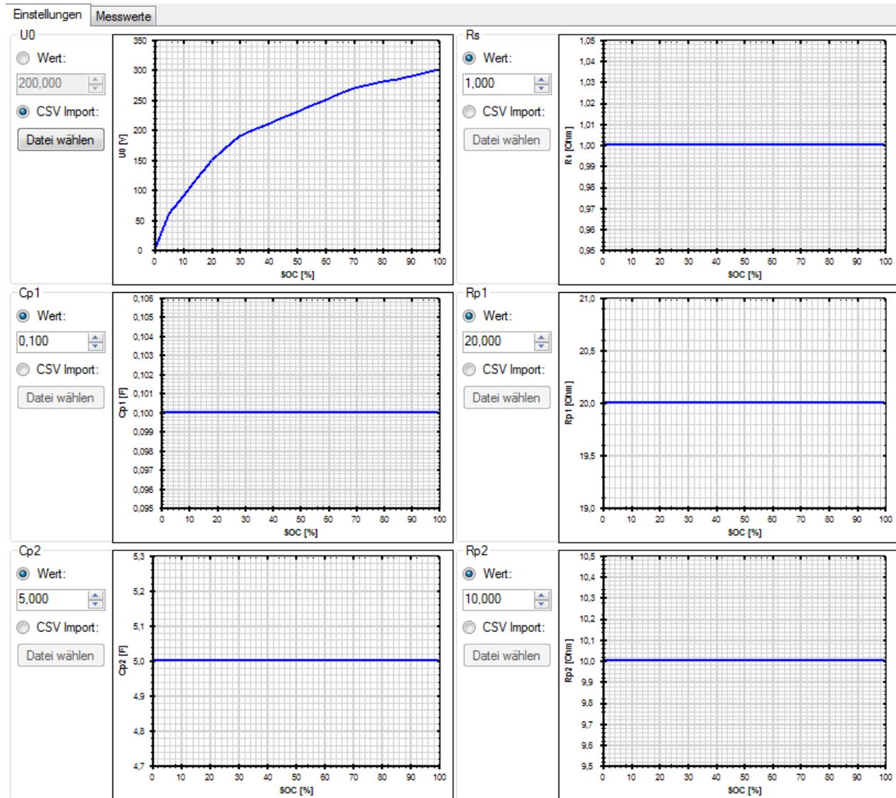
The input parameters of the battery characteristic in relation to the state of charge:
