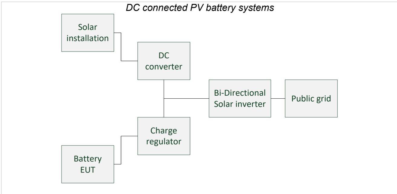
The PV Simulator PVS can operate either as generator / simulator of the PV installation or as battery simulator.
