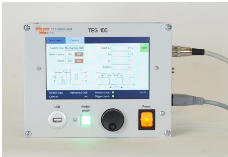
Fig. 14: TEG 100 control unit
