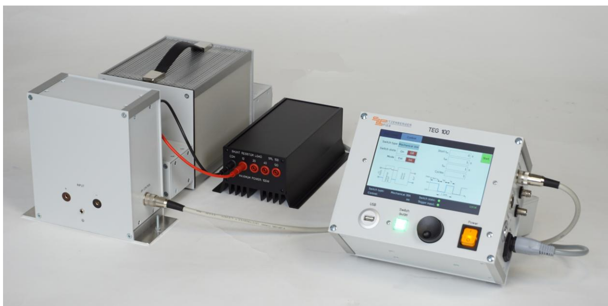
Fig. 11: Sample transient emission test setup with mechanical switch
