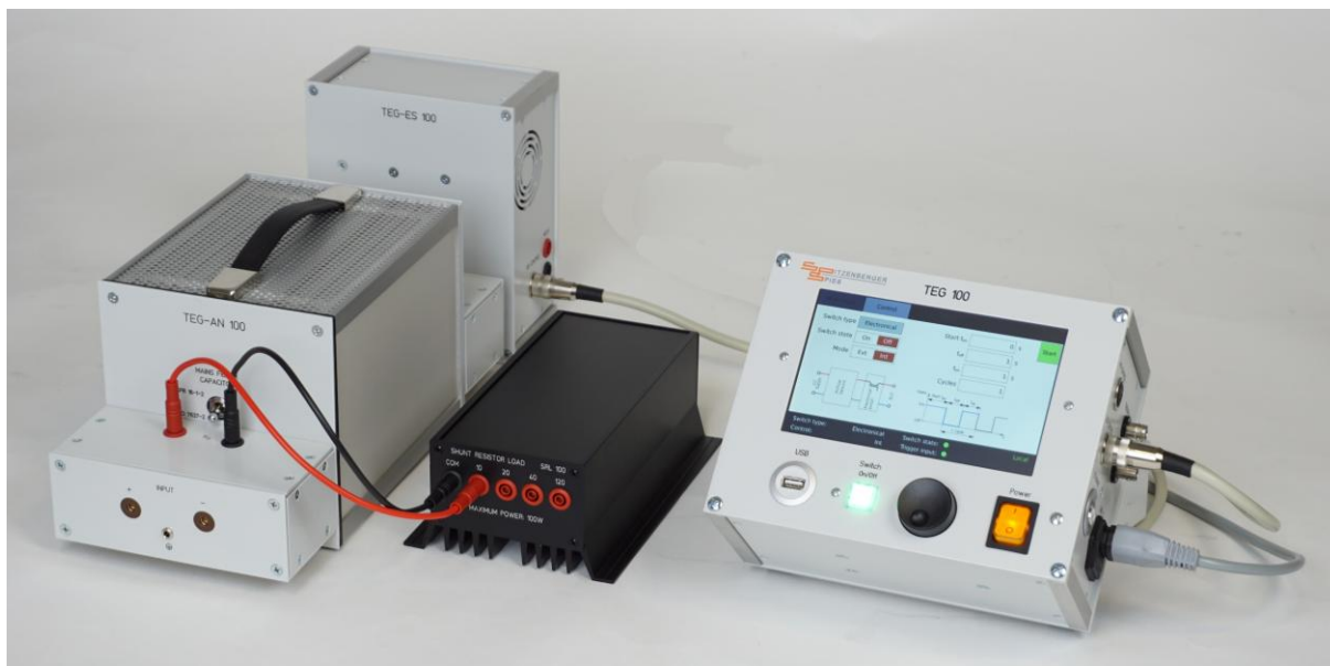
Fig. 13: Sample transient emission test setup with electronical switch
