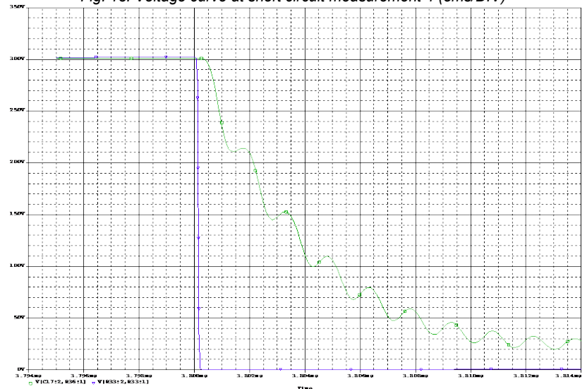
Fig. 14: Voltage curve at short circuit measurement 4 (0,5μs/DIV)
