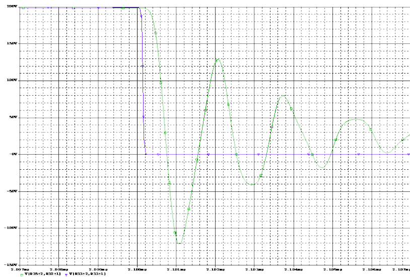
Fig. 7: Voltage curve at short circuit measurement 1 (1μs/DIV)
